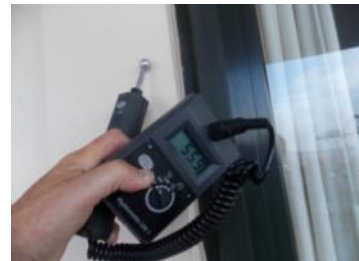
Dielectric constant moisture meter
